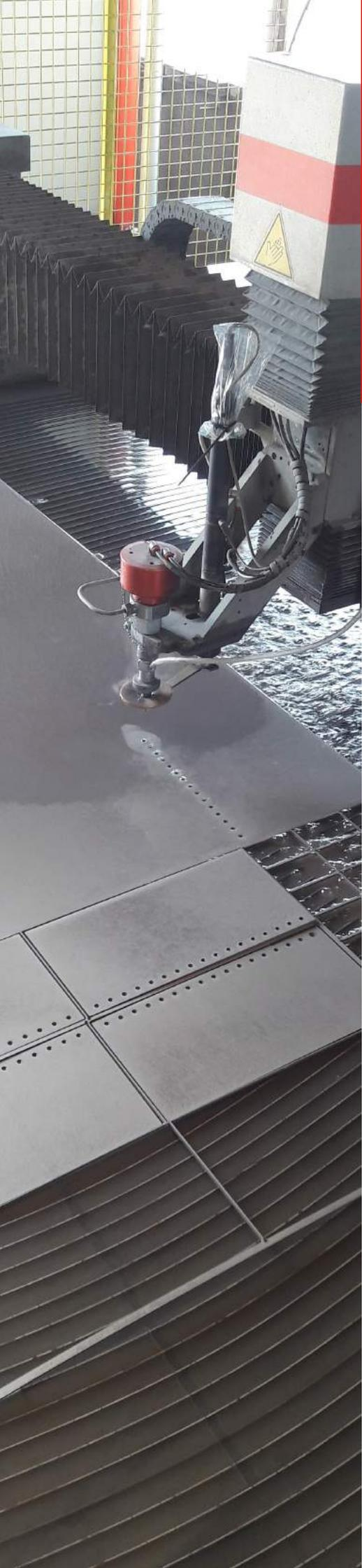
A photograph of a waterjet cutting machine in operation. The machine's head is positioned over a large metal sheet, which is being cut. The cutting process is creating a series of small holes and a narrow slot in the metal. The machine is mounted on a grid-like base. In the background, there are safety barriers and a control panel with a warning sign.
